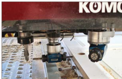
CNC Router cuts the door's contours and mortises the hinges and bores
