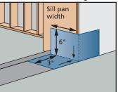
6. Seal back corners of sill pan with sealant.
