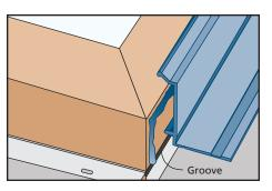
Inswing/outswing doors will need a strip of self-adhered flashing applied over the dead bolt or latch hole on the exterior side of the frame as shown.
