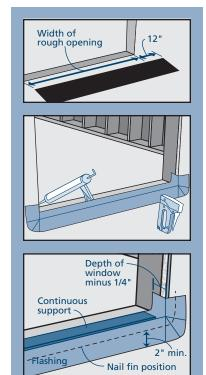
10. Align the shimming on the sill flush with the exterior and centered between the side jambs. If installing a mulled unit, shim under the mull joint(s) and tack into place or secure with sealant.
