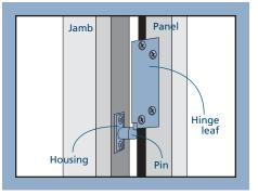
Slide the top hinge leaf onto the upper pivot and align the top of the panel with
