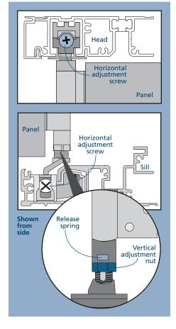
One rotation will provide approximately 1/16" adjustment. Right will raise and left will lower the panel. Adjust as necessary to achieve a consistent reveal across the opening.
