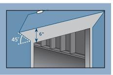
recommend installing a drip cap because this integrates the building wrap and drip cap to protect the structure and the product from incidental water.
