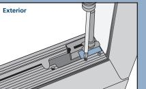
Apply the aluminum sill cover plate on top of the lower pivot hinge and secure with two #8 x 3/8" screws.
