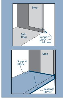
that requires multiple pieces, begin from the exterior and work in, overlapping the previous piece (shiplap method). Run a bead of sealant on both ends where the blocking material meets the jambs.
