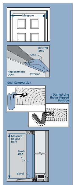
and cut jamb stops to fit. At the head, trim the jamb weatherstrip to fit around the head weatherstrip. Secure with five of the provided 6d galvanized finish nails on each jamb.
