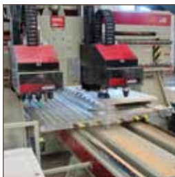
KOMO routes the door contours and mortises the hinges and bores.
