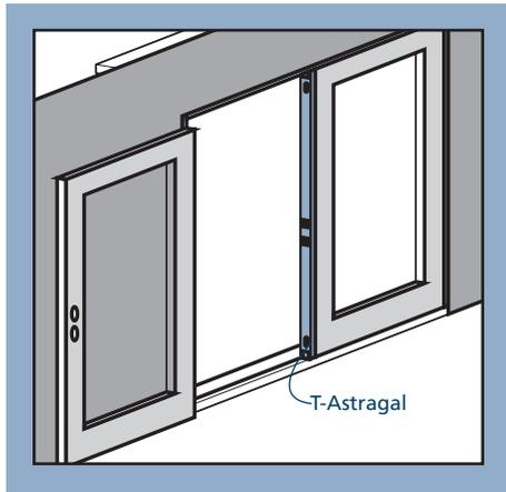
2. With the inactive door closed, mark where the flush bolts touch the head jamb and sill cap.
