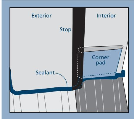
3. Apply sealant at the bottom where the sill meets the frame on both sides. If a sill extender is used, apply a bead of sealant between the sill and the extender. Apply sealant around any mulls at the intersection of the mull and door sill.
