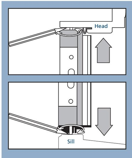
3. Drill 3/8" holes (1" deep) at these spots and apply the strike plates (provided) to the sill cap and head jamb as shown.
