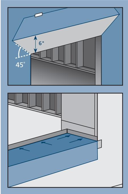
6. Cut two pieces of self-adhered flashing 6" wide by the sill pan width + 3" long.
