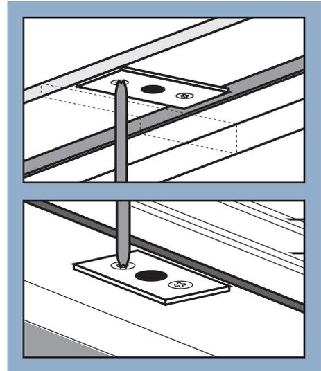
4. With the inactive door closed, mark the head jamb weatherstrip with a sharp utility knife at the edge of the T-Astragal where it touches the weatherstrip. Open the inactive door and cut through the weatherstrip so that when the door is closed the weatherstrip clears the T-Astragal.
