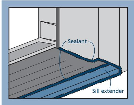
4. Apply sealant around the outside of the door unit between the siding and brickmould and between the brickmould and the jamb. Also apply sealant between the jamb sides and the threshold. Run a bead of sealant, leaving 1" gaps every 2', along the front side of the threshold where it meets the slab/rough opening.
