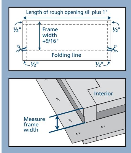
5. For step-down landings, cut 1/2" in at this line on both sides of the sheet material.
